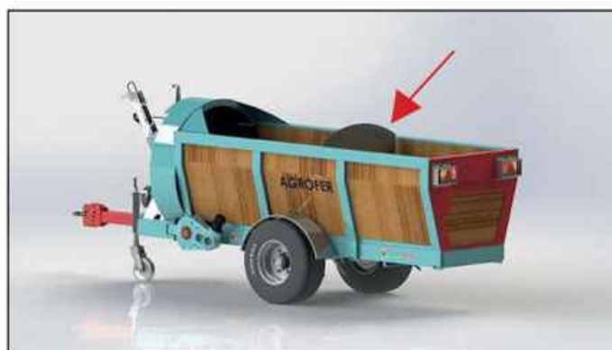
Wall for advancement on chain
